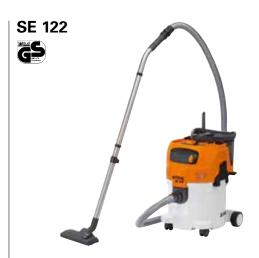
**1.5 kW, 250 mbar, 3,700 l/min.** With multiple filter system, integrated accessories box and suction tube holder. Wet and dry vacuuming options, filter cleaning, filter element/bag, castors with locking brakes, stainless steel handle with quick-release coupling.
