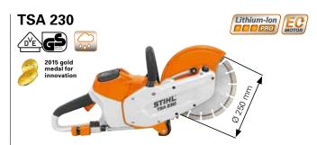
Easy-to-manoeuvre battery cut-off machine for 230 mm cutting wheels. Suitable for indoor and outdoor use, up to 70 mm cutting depth, water connection with ball valve and hose coupling for wet cutting, spindle lock, maintenance-free belt drive. Weight: 3.9 kg <sup>①</sup>.
