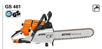
**76.5** cm³, **4.3** kW/5.8 hp, **7.6** kg<sup>©</sup>. Handles like a chainsaw, with the power of a cut-off machine. Side-mounted chain tensioning, STIHL anti-vibration system, water connection, decompression valve, STIHL ElastoStart, wear-resistant starter cord, HD2 filter, tank with bayonet fuel cap for upright refuelling, 2-MIX engine.
