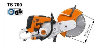
**98.5 cm³, 5.0 kW**/6.8 hp, **11.7 kg**<sup>①</sup>. Most powerful cut-off machine for 350 mm cutting wheels. The cut-off machine is perfectly suited to use at full cutting depth and also on the FW 20 cart. Equipped with decompression valve and STIHL ElastoStart for effortless starting and the long-life air filter system. Economical 2-MIX engine.
