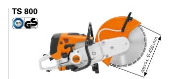
**98.5 cm³, 5.0 kW**/6.8 hp, **12.7 kg**<sup>©</sup>. STIHL cut-off machine for 400, 416, 418 mm cutting wheels. Attains the maximum cutting depth of 145 mm, reduced weight due to magnesium guard. Also perfectly suited for carrying out separating cuts on the FW 20 cart. Equipped with decompression valve and STIHL ElastoStart for effortless starting and the long-life air filter system. Economical 2-MIX engine.
